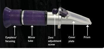
The Kamco refractometer 402 has been designed to give a rapid indication of the level of concentration of Freezbreaker and other glycol based antifreeze compounds. Both the concentration, and the likely degree of protection are indicated.
